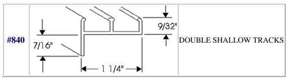
ALL TRACKS ARE .062 THICK 6063-T6 EXTRUDED ALUMINUM ALL TRACKS ARE DESIGNED FOR USE WITH 7/16" THICK FRAMES
