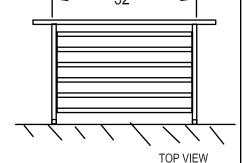
COAT RACK: 16 10HK molded, double prong polycarbonate hooks, available in 9 colors, locked in either silver or bronze aluminum slats, secured to die cast aluminum brackets. Brackets are finished with black powder coating.
